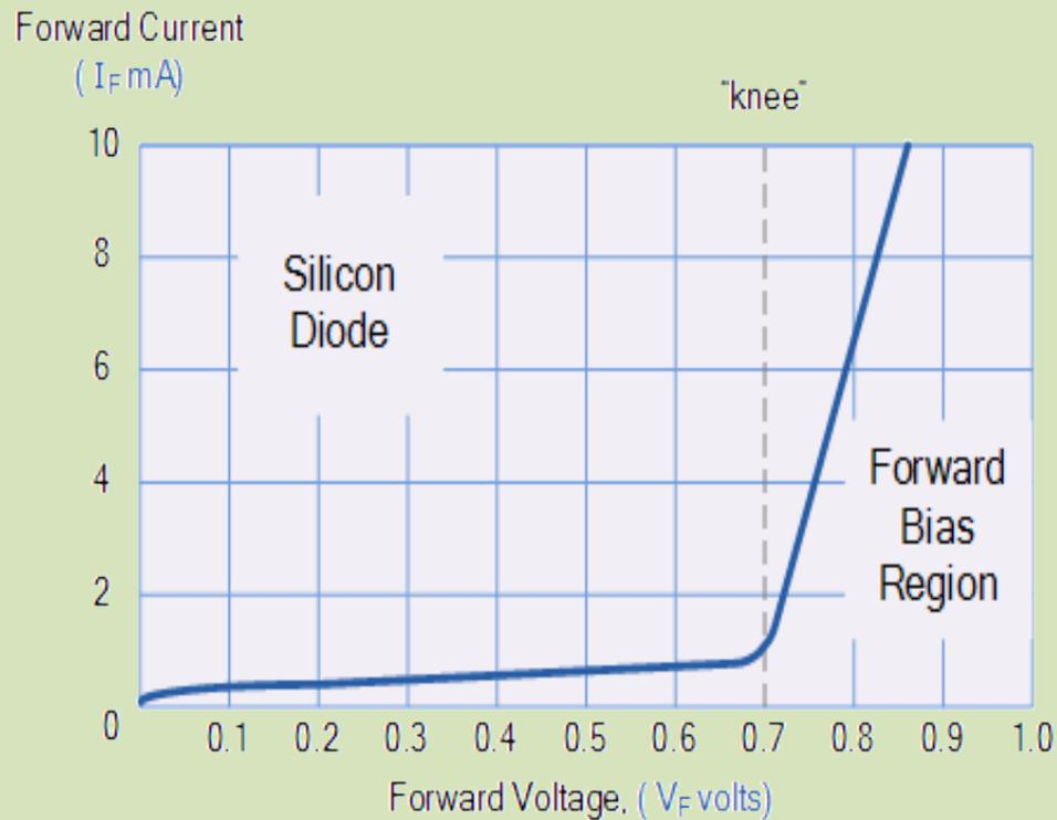
The application of a forward biasing voltage on the junction diode results in the depletion layer becoming very thin and narrow which represents a low impedance path through the junction thereby allowing high currents to flow. The point at which this sudden increase in current takes place is represented on the static I-V characteristics curve above as the “knee” point.
